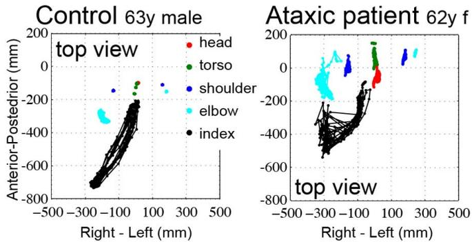
Fig. 1. Digitized SARA (nose-finger test) with Kinect v2. In contrast to low (a few cm) resolution of conventional SARA, it is possible to evaluate body movement with 1-mm resolution using our digital-SARA. It should be emphasized that most clinical evaluations focus only on movement of small body parts (e.g. index finger: black dot), while our system provides a precise description of both individual body parts and the whole body.
