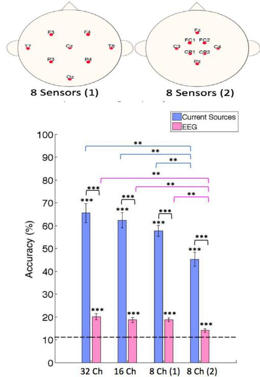
Figure 4 – Classification accuracies for four types of EEG sensor configurations. \*\*\*  $p < 0.001$ , \*\*  $p < 0.01$  and \*  $p < 0.05$ .
