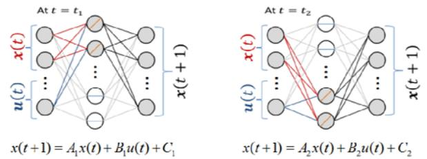
Fig. 2. A neural network for learning the forward dynamics of the muscular-skeletal humanoid upper-body. It has a restricted linear unit (ReLU) as activation function of the middle layers. The ReLU enable to pick the activated unit at the time, and derive linear state equation.
