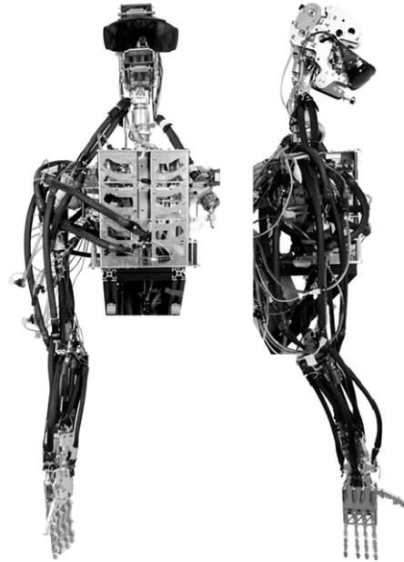
Fig. 1. Muscular-skeletal humanoid upper-body. (The robot is equipped with 28 artificial pneumatic muscles and 1 spring. It has shoulder, elbow, an wrist joints, and a 1 DOF hand. The muscular structure is similar to that of a human.)
