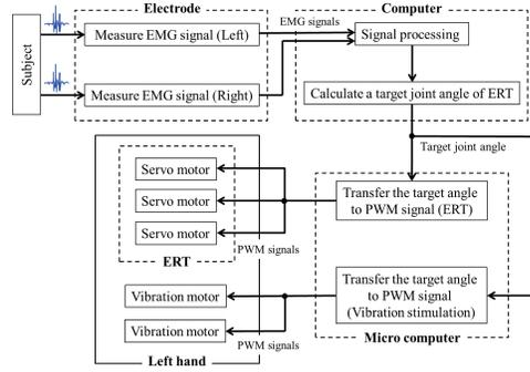
Fig. 1. Overview of the system and system architecture.
