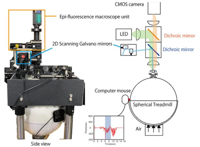
Fig. 3. Galvo mirror controlled photoactivation system with spherical treadmill system.
